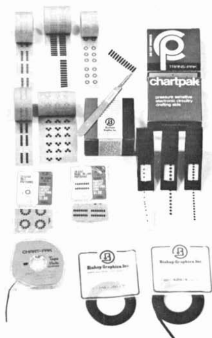
Drafting aids used in preparing the artwork for the printed-circuit board.
